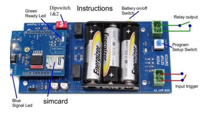
Please make sure you disconnect the power when you fit the simcard. Then slide the simcard into the holder making sure that the clipped corner of the simcard lines up with the clipped corner of the simcard holder as seen in the image above.
