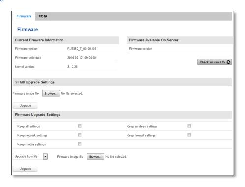
**STM8 Firmware** –it is responsible for sleep mode functionality and signal strength leds.
