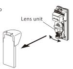
②Adjust the angle of the sensor with vertical adjustment screw by looking through the viewfinder. Continue adjust until the center of the reflector can be seen in the middle of Vertically ± 5 the viewfinder as shown on Vertical adjustment screw the right.
