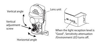
When the direction of the optical axis roughly matches the reflector, a beep sound begins which changes according to the light reception level as below.
