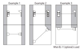
Install the reflector directly, facing the front of the optical unit as much as possible.
