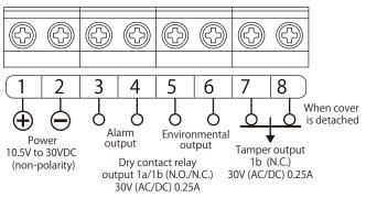
Current consumption (Max): 200 mA (DC10.5V) 160 mA (DC12V) 80 mA (DC24V)
