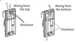
⑤ After wiring is completed, adjust alignment, attach cover and check operation.
