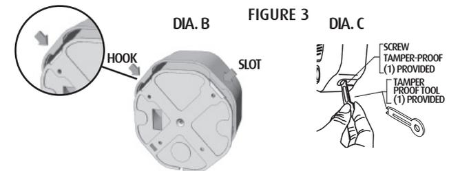
VIEW SHOWING HOW TO FIX THE COVER TO THE BASE
